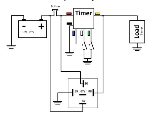
Alternatively, timer can perform the same function without the relay. The timer should be set to function #2 and trigger to #4. The circuit consumes 4ma during power off state. If the circuit is not battery powered or there is no concern regarding 4ma current drain by the timer, then this circuit is preferred as it does not require a relay.
