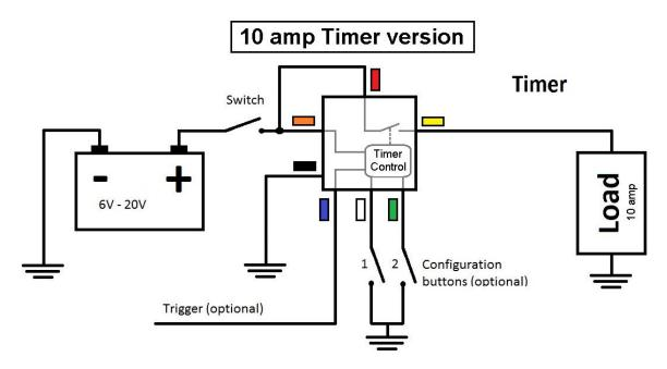
Separating power for timer circuit and timer output provides greater application flexibility. It allows for the timer to be connected directly to the power supply battery but control the timer function with a lower power signal like car or motorcycle ignition wire. With ignition OFF the timer has zero standby current consumption which is great for battery powered applications. With the ignition ON timer performs the required timer function.
